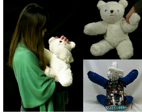
Figure 1: An example of touching interaction and appearance and inside of the cuddly robot. The cuddly robot is soft to the bone.
